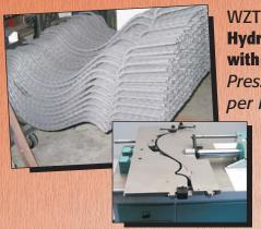
WZT24 **Hydraulic Bender** with Belly Picket Die Press 150 per hour!
